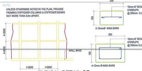
6 TYPICAL DETAIL OF STIFFENER BEAMS & COLUMNS
